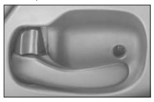
To lock a door from the inside, push the manual lock lever forward. To unlock a door, push the lever rearward.
